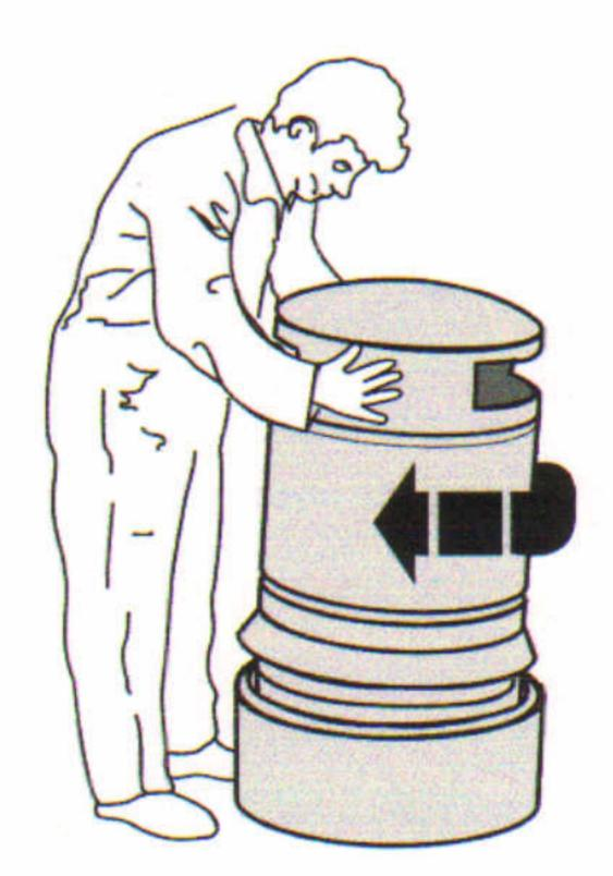
4 Lift bin body over liner and drop onto plinth to lock.
